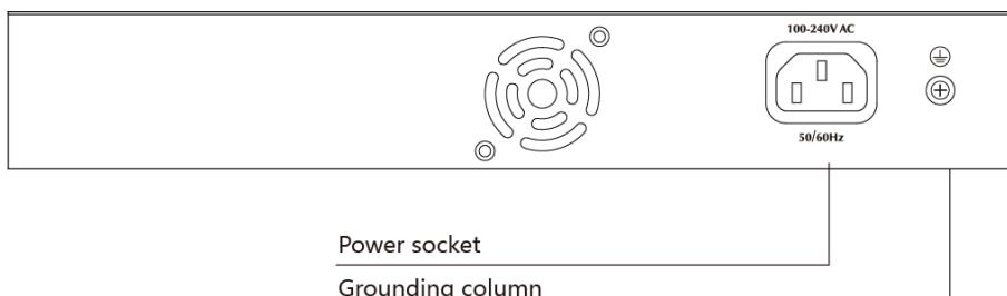
The 24GE+4G SFP Switch have AC power connector, AC input range 100-240V, 50/60HZ, a grounding screw holes, as shown below:
