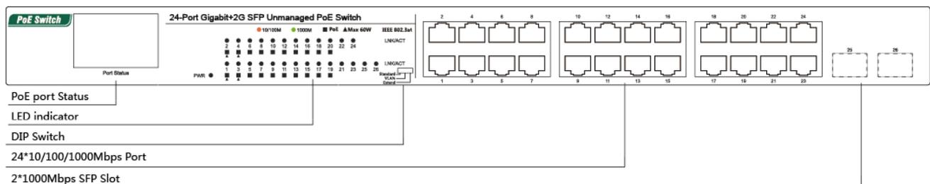
24\*10/100/1000Mbps Adaptive RJ45 port,in which 1-4 PoE port output power up to 60W,5-20 PoE port output power up to 32W,21-24 ports without PoE
