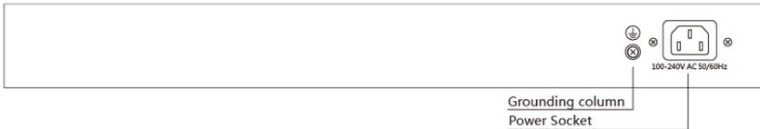
**Note:**This device relies on the separate protective earthing terminal. The device installation shall be permanently connected to building earth by a skilled person. The device shall be intended to be used in a location having equipotential bonding(such as a telecommunication centre, a dedicated computer room, or a restricted access area).
