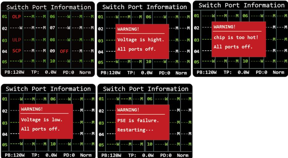
Not only such visible on the basis of three generations in the second generation increases the color logo, according to the menu button, switch mode, bandwidth display and warning, PD type, PSE power fine-tuning and priority, PoE port switch control, LCD switch. Enhance the LCD viewing angles, smart fan control, language selection and the function of the factory Settings, in turn, as shown in the figure below: **See the operation instructions of the screen concretely.**
