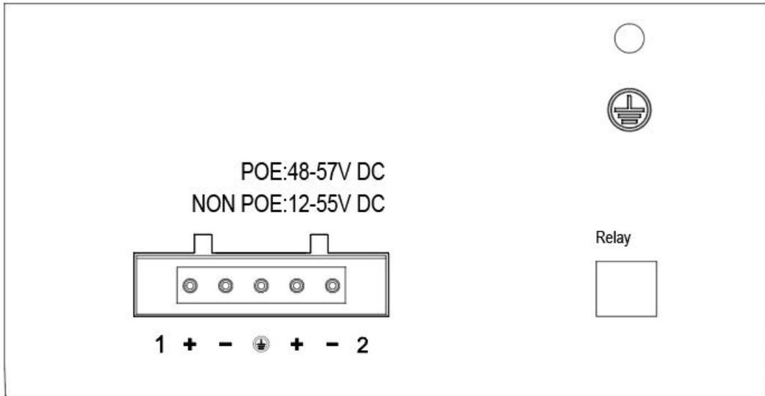
Figure 3-2 8-Port Gigabit + 4G Combo Switch side panel
