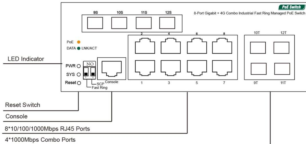
Figure 3-1 Front panel of the 8-Port Gigabit + 4G Combo Switch
