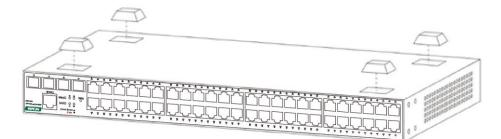
Figure 3-1 Desktop Installation Diagram
