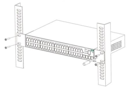
Figure 3-3 Diagram 2 of rack installation
