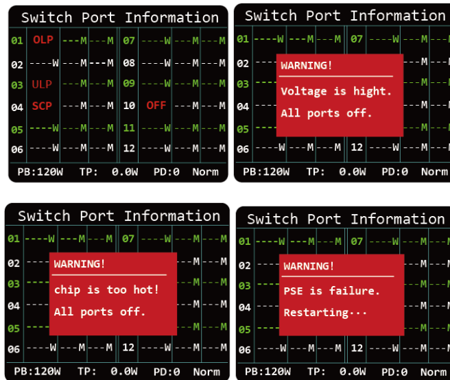
Figure 2-3 Schematic diagram of LCD screen working condition
