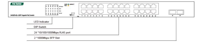
**Default:** The factory default mode is used when the CCTV is turned off. In this mode, it is equivalent to a common switch. Ports 1 to 26 can communicate normally.
