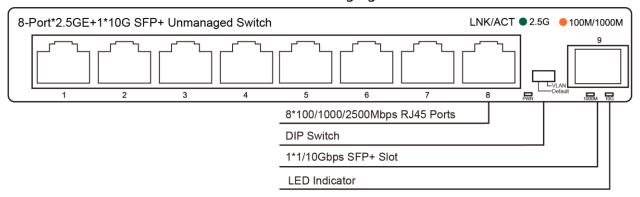
Figure 2-1 Switch front panel diagram
