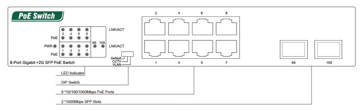
**Default:** indicates the factory Default mode. In this mode, ports 1 to 8 can communicate with each other properly. **VLAN:** In VLAN isolation mode, ports 1 to 8 and 9/10 on the switch are divided into independent VLAN. Ports 1 to 8 can only communicate with ports 9 and 10. Ports 1 to 8 cannot communicate with each other to ensure network security. In this mode, connect 9/10 to the central switching device.
