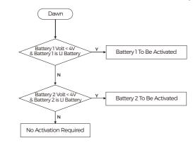
7.3 Switching logic between battery 1 and battery 2 during abnormal operation. (battery with load during operation) (take 12V system as an example)
