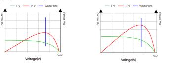
7.7.3 The effect of temperature on light. (the higher the temperature, the lower the open circuit voltage, but the overall power is almost the same)
