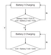
7.4 Switching logic between battery 1 and battery 2 during normal
