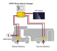
**6.3 The alternator is connected to the external input port of the controller**. (this application is similar to the adapter or power supply directly connected to the external input port)(DC input only)
