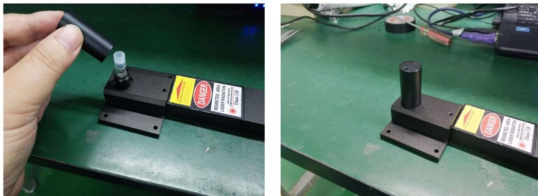
Fig 2 Fluid sample cell (Liquid chromatography bottle) (Optional)
