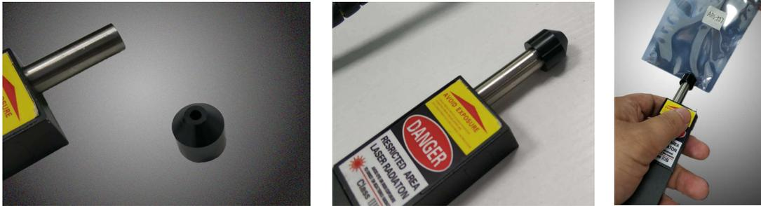
Fig 2 Solid, powder measuring probe
