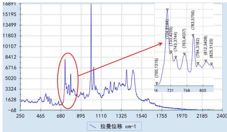
Fig.2.3 Raman spectrum of petrol 93#, the vibration mode 723/732/742cm<sup>-1</sup> can be resolved.
