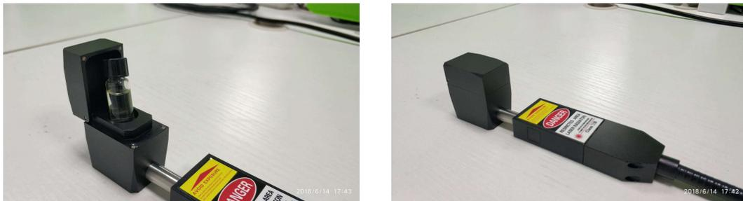
Fig 1 Fluid sample cell (Thermo bottle)
