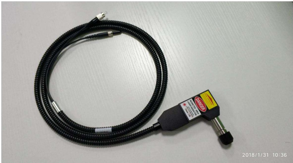
Fig 5 Raman probe gun (optional)
