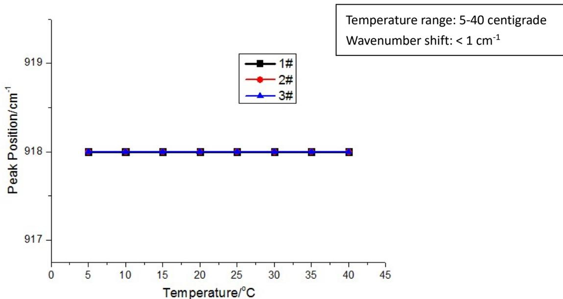
Fig. 3.1 Wavenumber shift results testing from 5 °C to 40 °C of fives ATR3000 portable Raman spectrometers
