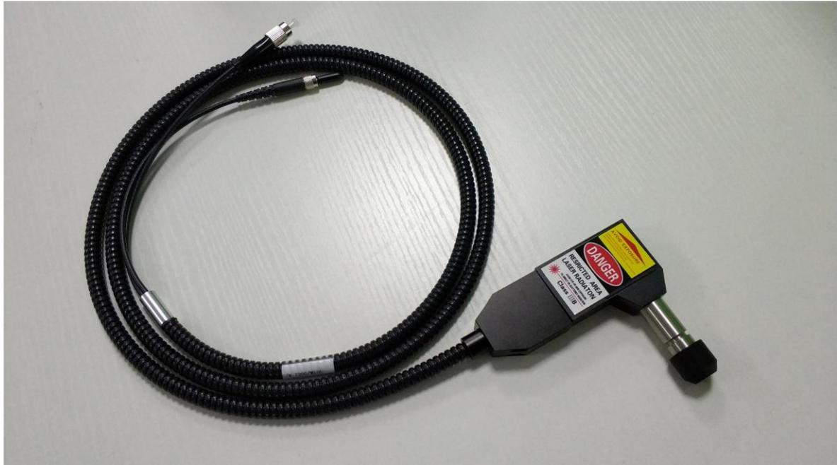
Figure 4 ATR20107, the gun-type Raman probe. The parameters is the same as ATR20105
