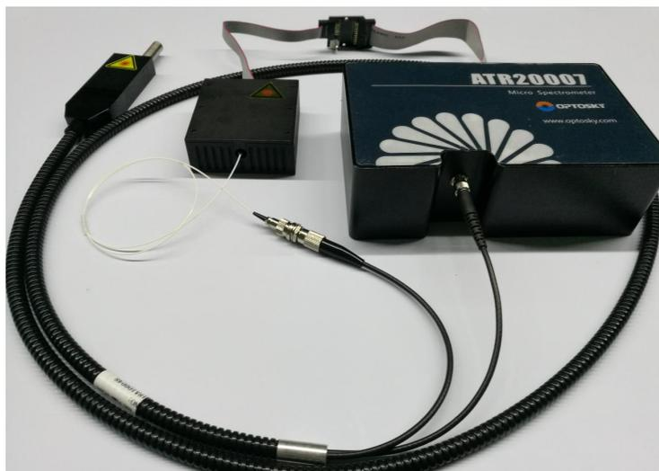
Figure 3 Raman system physical picture
