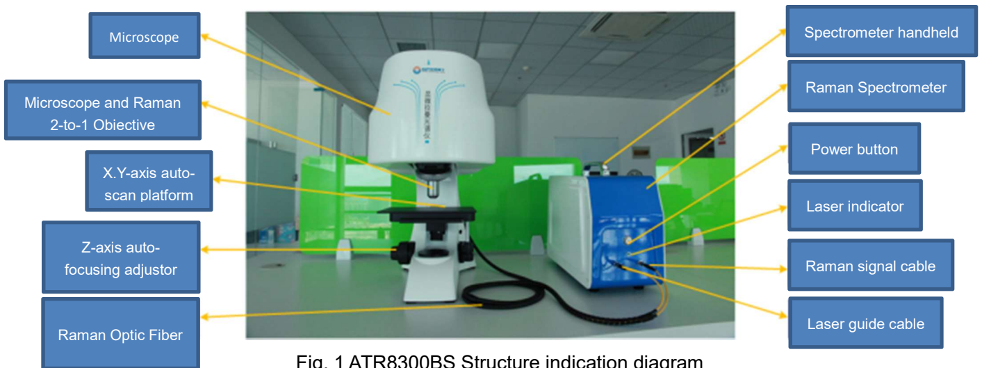
Fig. 1 ATR8300BS Structure indication diagram
