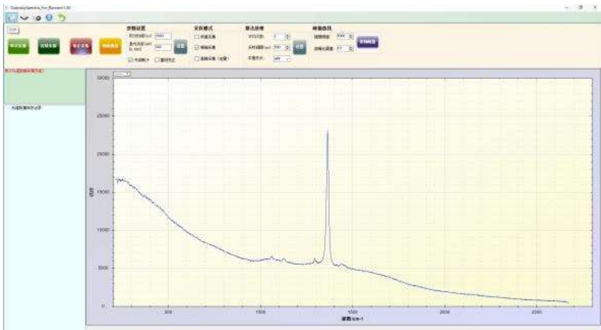
Fig 6 ATR8300BS measure boron carbide (PN) spectra (200mW, integration time: 2S)
