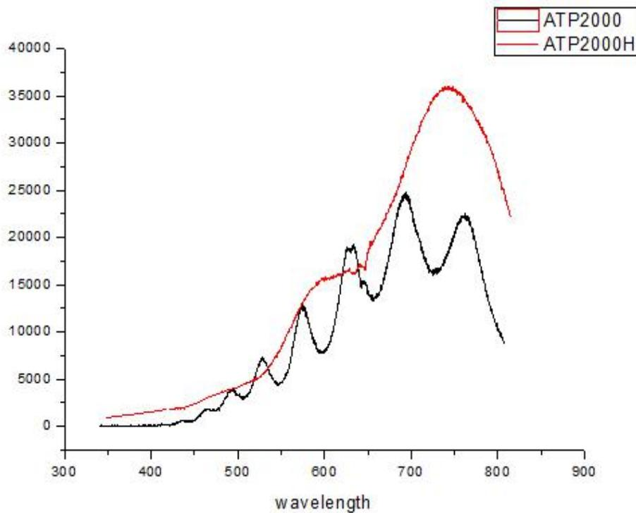
图 2 The sensitive of ATP2000P/ATP2000H (Red) vs ATP2000 (Black)
