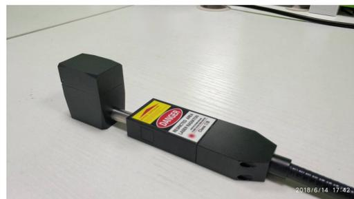
Fig 1 Liquid sample cell (similar to Thermo)
