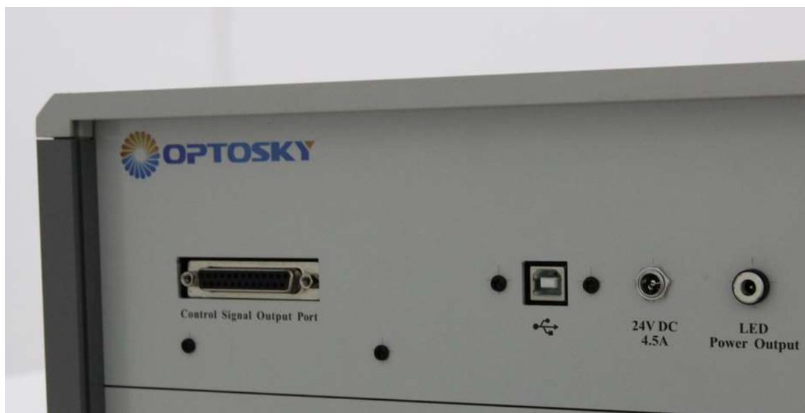
Fig 12 Simple interface: Raman spectrometer: power socket +USB2.0 connector
