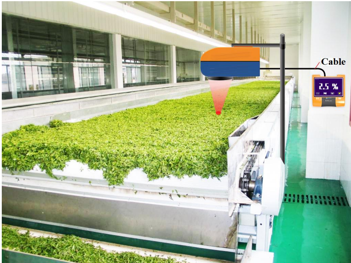
Figure 1 Application of GY1000 Online Infrared Moisture Analyzer
