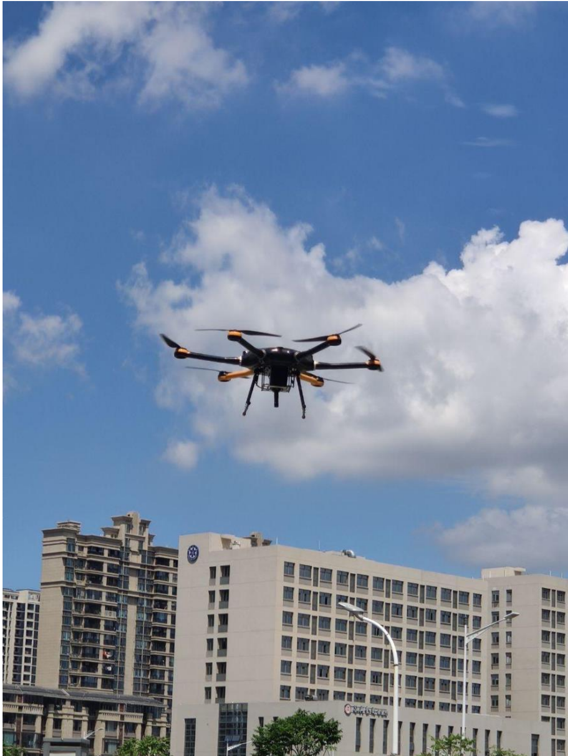
Fig 2 Flight Experiment of UAV-borne Methane Leak Inspection System (Location: Xiamen Rare Earth Research Institute, Chinese Academy of Sciences)
