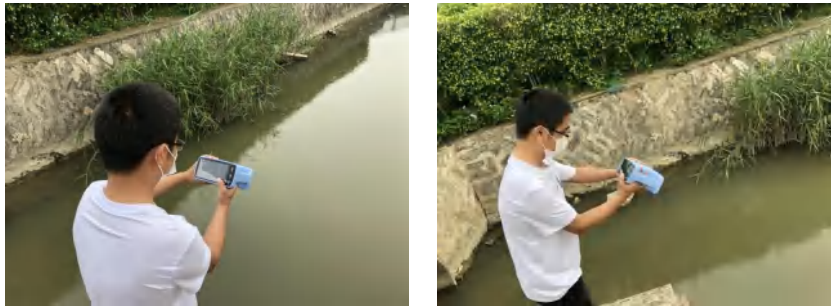
Fig 9 ATP9100 measure spectra of sky, lake and red tide
