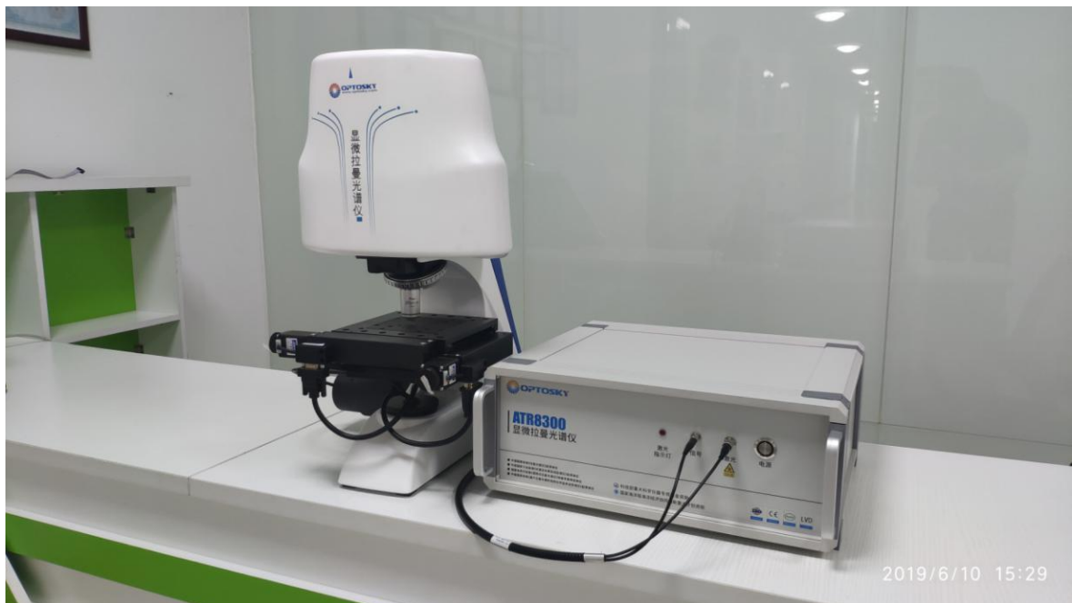
Figure 21 High transmittance objective for Raman signals. Objective focal length up to 8 mm.
