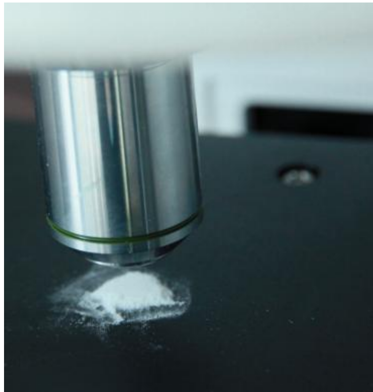
Fig 11 Raman signal high through put objectives with focal length up to 8mm;
