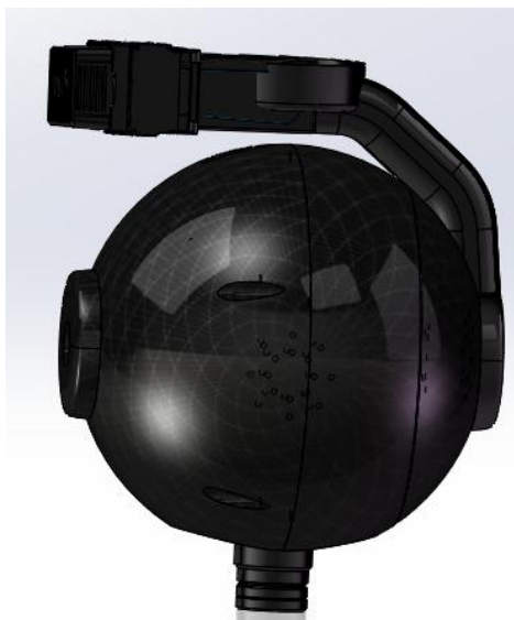
Figure 5. Oil pollution detection system with fluorescent scanning imaging
