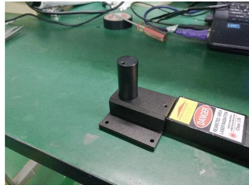
Figure 2 Liquid sample measuring cell (LC bottle, micro volume)
