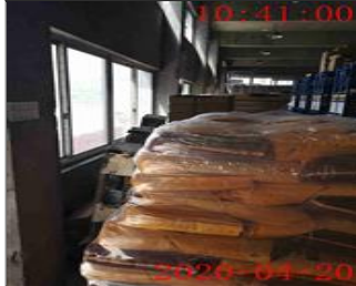
Photo of non-conformity Goods were directly leaned against the wall and post.jpg
